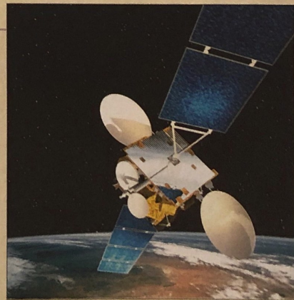
▲ Figure 11-9 On this artist's drawing of a communications satellite, the large blue panels contain the solar cells.
