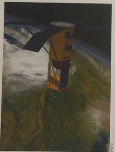
Figure 2-61 The SeaStar satellite with the SeaWiFS instrument. The SeaViewing Wide Field-of-View Sensor (or SeaWiFS) instrument is part of the SeaStar satellite. The SeaStar is an excellent example of a satellite used by oceanographers. It provides information on subtle changes in ocean color, which indicate the presence and concentration of microscopic marine plants called phytoplankton. The greener the water, the more phytoplankton is present.
